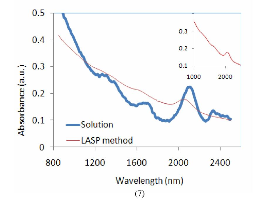
The UV- absorption spectra of the 200 nm thick film and colloidal solution of PbSe QDs with average particle sizes of 9.5 nm is shown in Fig. 7 The first, second and the third quantum levels were observed in both samples. In addition, the blue shift in the absorption peaks corresponding to decrease in particle size is also noticeable. Lower intensities are observed due to the small absorption length in the film in comparison to the solution.
