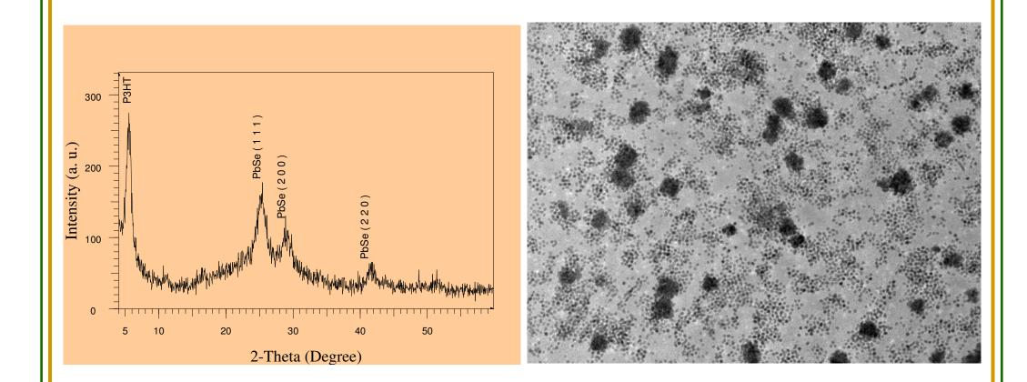
Peaks of XRD pattern confirms the formation of P3HT polymer and the PbSe NC in the film.TEM imaged shows the initial formation of P3HT polymer and the PbSe NC on the film. It provides a good evidence of uniformity of PdSe Qds in the hybrid structure.
