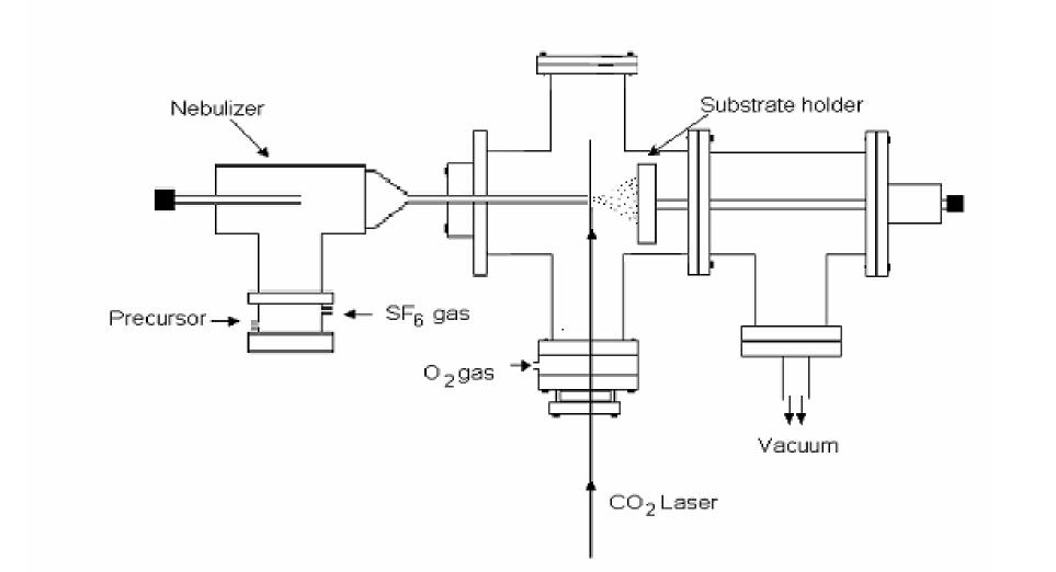
This laser-assisted spray (LAS) process for the growth of nanoparticle films offers two main advantages over the more conventional spin-coating and drop-casting methods: (1) the surfactants are burnt-out prior to deposition and thus QDs form intimate contacts between QDs and QDs and the host materials, (2) nanoparticles are sprayed uniformly over the substrate preventing local segregation of QDs.
